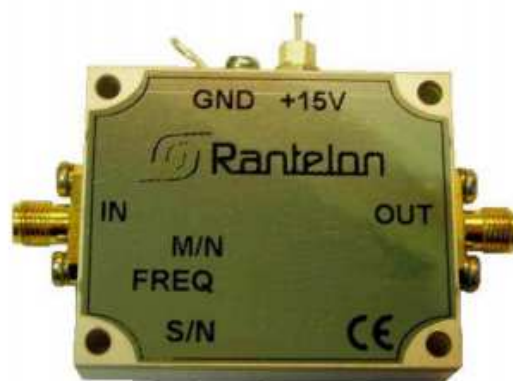
KA1907 mechanical enclosure.
