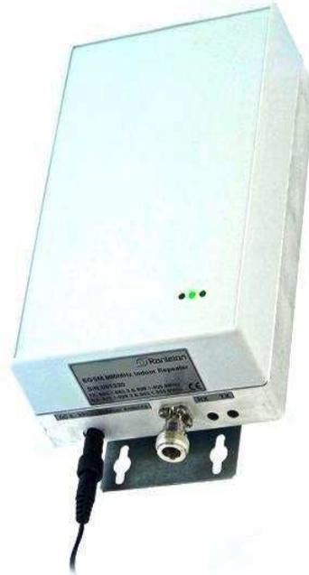
Figure 1: Repeater GR1831 front view
