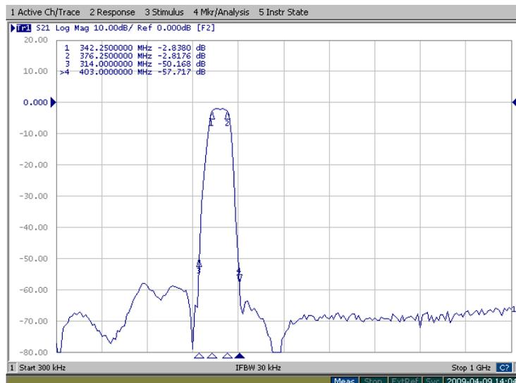
Figure 3: FB-359.25M transfer function 300kHz-1GHz band.
