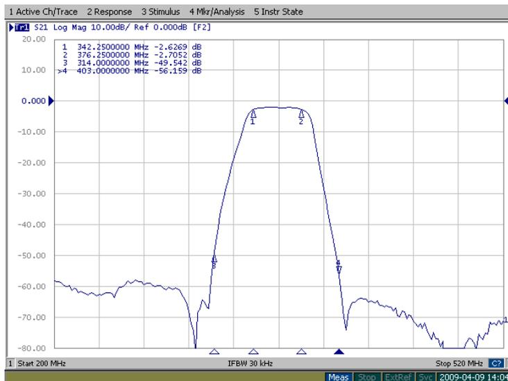
Figure 2: FB-359.25M transfer function in 200-520MHz band.
