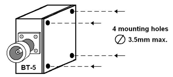
BT-5 can be mounted through four 3.5mm diameter holes, using suitable screws (as example M3x30) or other proper tools.
