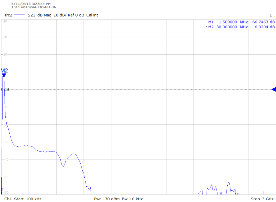
Figure 4: ASJ8-1 transfer function curve up to 3GHz
