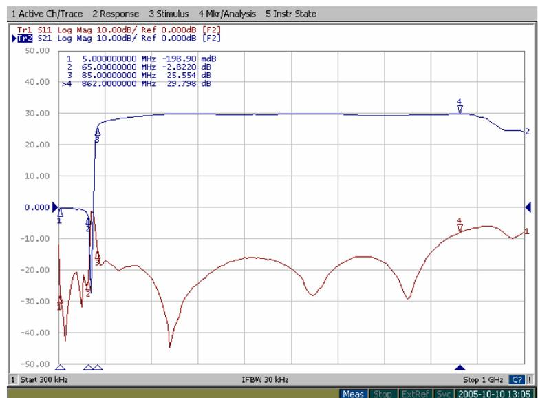
Figure 1. Amplifier transfer function S21
