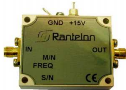
KA1303-LEM mechanical enclosure
