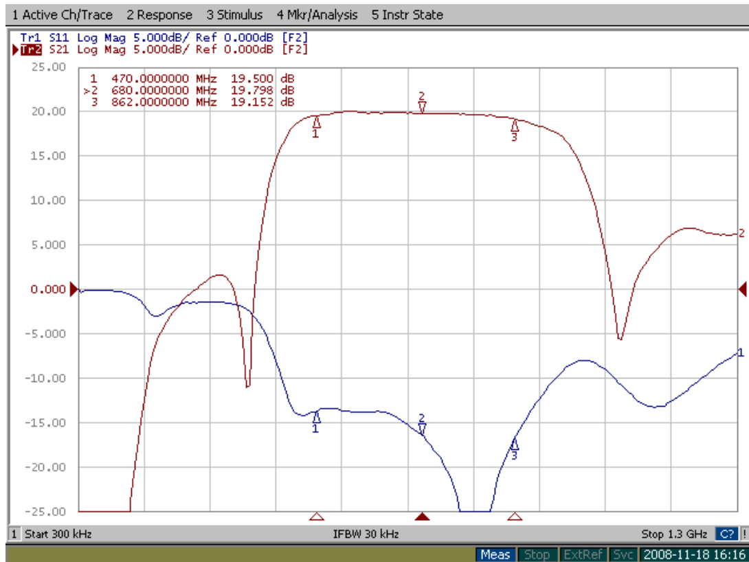
Example of ZA-20 input return loss (-S11) and transmission (S21) curves.
