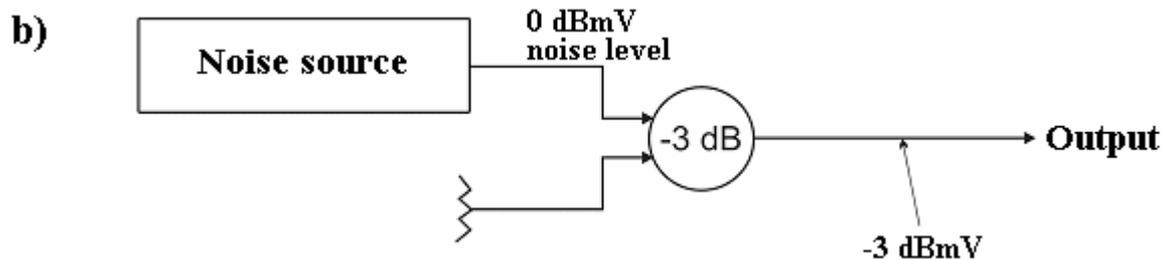
In diagram *b* one of the noise sources is disconnected. Half of the noise power will heat the resistor inside a splitter and another half reaches the splitter output, causing the signal level in output to become -3 dBmV. Therefore the output noise power is 3 dB less than input noise power.
