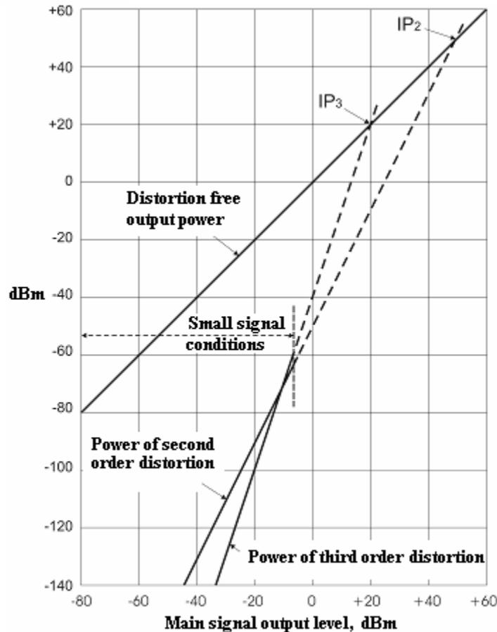
An amplifier is always intended to work at much lower frequencies than  $IP_2$  or  $IP_3$ . Those parameters are still widely used to describe amplifiers, since the values of  $IP_2$  or  $IP_3$  may be well used to estimate the distortion level also in small signal conditions. The greater the  $IP_2$  and  $IP_3$ , the lower the distortion products and the higher the quality of CATV signal.
