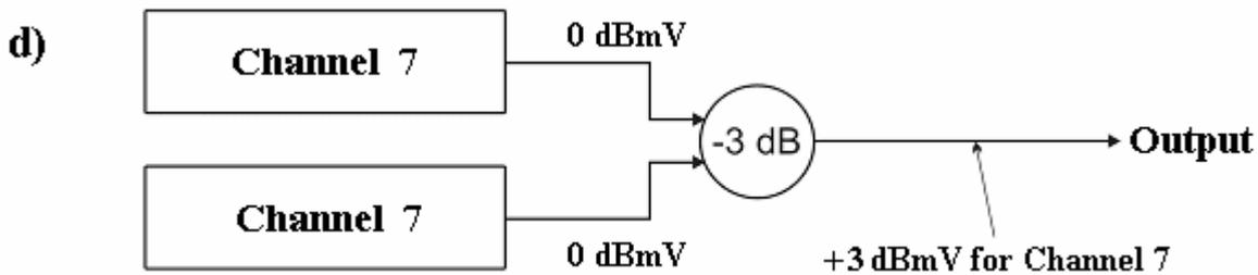
In diagram *d* there are two signal sources feeding the two ports of the splitter (functioning as a combiner) and both sources are tuned to the same frequency and phase. As the signals are identical, the voltage on the resistor inside the splitter is 0 and therefore the power loss is also 0. Thus, signal power in the splitter's output is 3 dB greater (2 times greater) compared to the input power.
