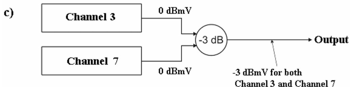
In diagram *c* there are two signal sources feeding the two ports of a splitter (functioning as a combiner) and each generator is operating on a different television frequency. As the signals are
