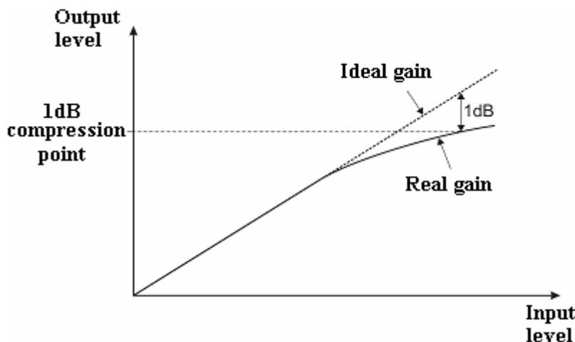
Parameters that describe nonlinear distortions are always given for small signal conditions, i.e. below 1 dB compression point. All CATV devices are intended to work below 1 dB compression point.
