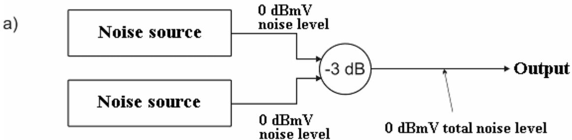
In diagram *a* there are two noise sources feeding a simple CATV splitter connected as a combiner. Assuming the splitter loss is 3 dB per port (half of the power), the noise entering the two ports at 0 dBmV will be attenuated at -3 dB, but will power-combine + 3 dB, causing the signal level in output to become 0 dBmV. Thus, the output noise power equals the input noise power.
