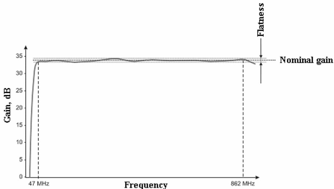
The flatness of amplifiers is typically  $\pm 1 \dots 2$  dB, in high quality amplifiers  $\pm 0.5 \dots 0.6$  dB.
