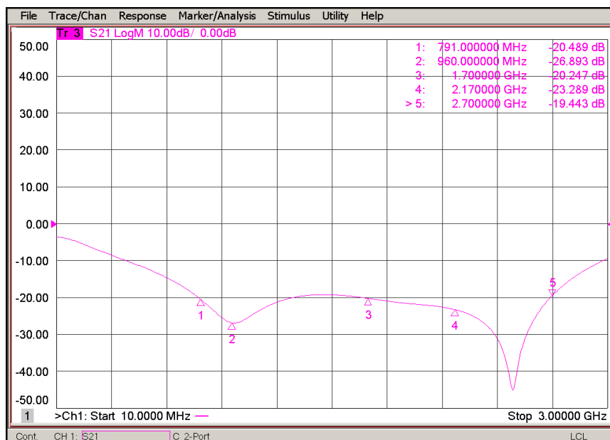
Example of isolation between output ports of PDW2-0727-50N.
