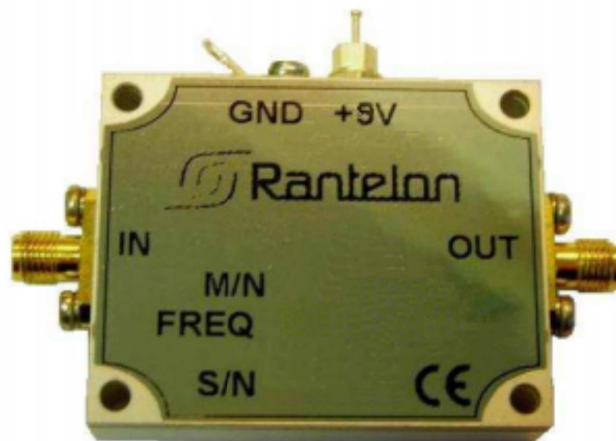
KA2506 mechanical enclosure.
